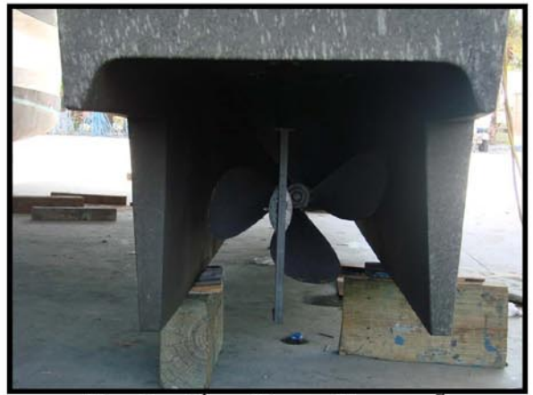
Protective Prop Tunnel
